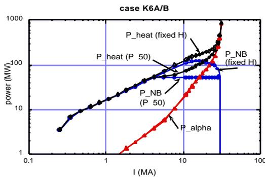
Fig. 5. Power input during startup on ARIES-ST.
