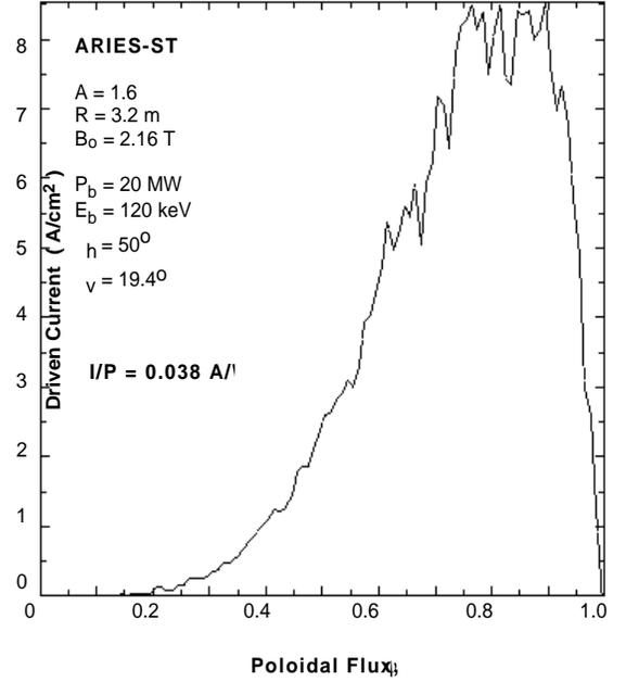
Fig.4. Off-axis neutral beam CD in ASRIES-ST.
