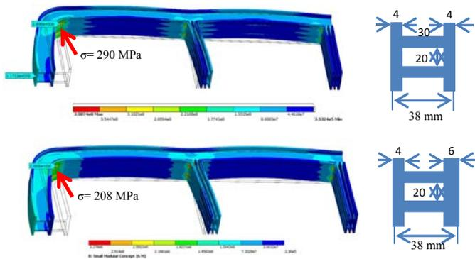
Fig. 18. Design solutions for an adapted 6 blanket modules/sector concept, Option 1 (top), Option 2: final solution (bottom)
