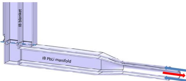
Fig. 10. Details of improved IB manifold design, Sectional view
