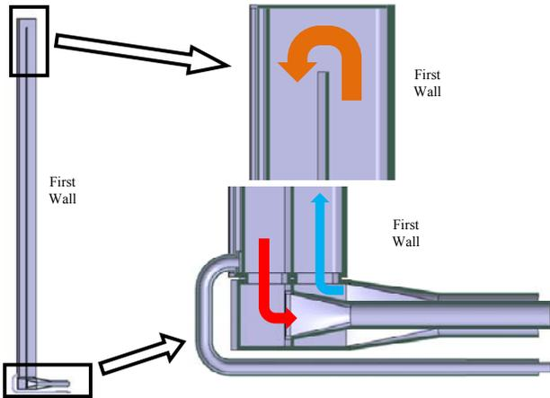
Fig. 3. First design for IB DCLL blanket module, R=8.5m; PbLi flow path
