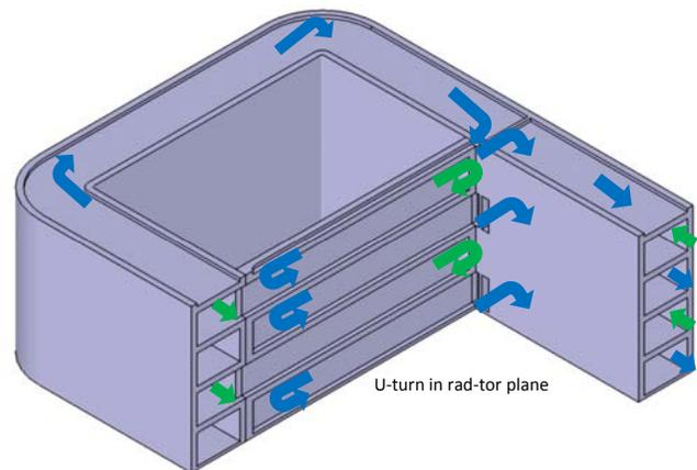
Fig. 5. Detail of helium flow path inside the modul walls
