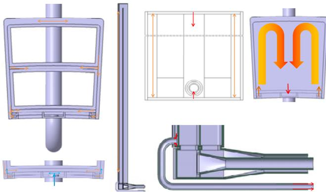
Fig. 4. First design for IB DCLL blanket module, R=8.5m; He flow path: Left: Inlet and SW/FW flow, Middle and Upper Right: Top/Bottom plate flow, Lower Right: Helium outlet flow
