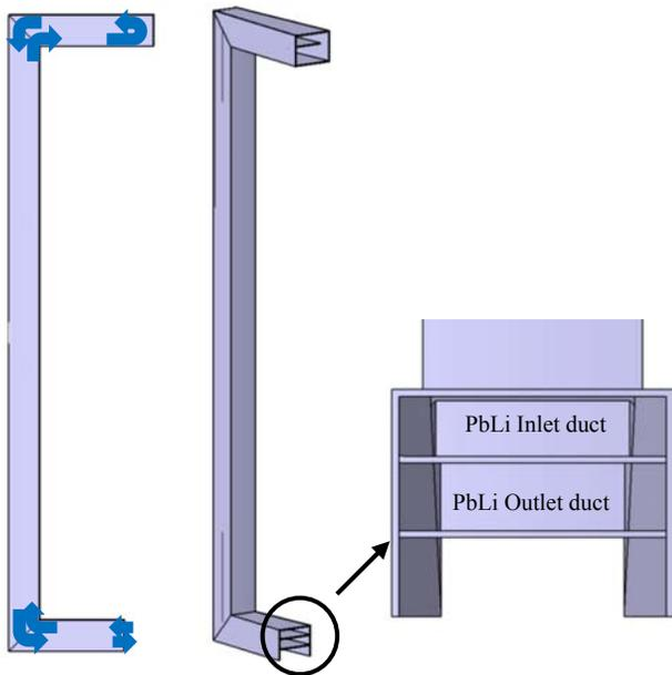
Fig. 7. Proposal of alternative C-shaped module, PbLi flow path, exemplarily for IB
