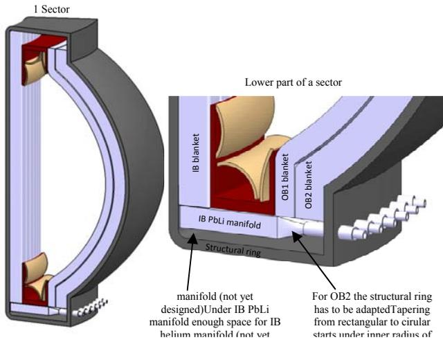
Fig. 9. Details of improved IB manifold design
