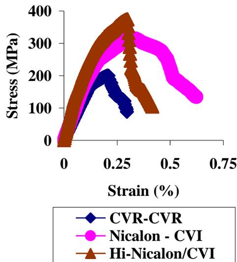
**Figure 8. Stress-strain curve for CVR-SiC/CVR-SiC composite.**
