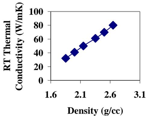
**Figure 2. Effect of composite density on thermal conductivity.**
