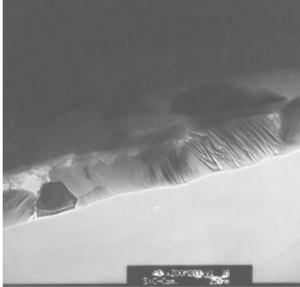
**Figure 5. TEM of CVR-SiC fiber.**
