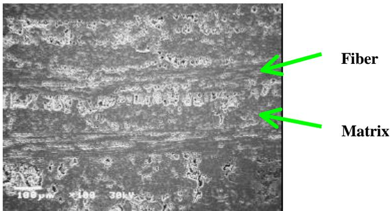
**Figure 7. Cross-section of CVR-SiC/CVR-SiC composite.**
