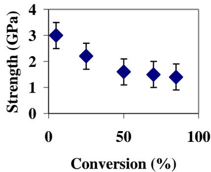
**Figure 3. Single fiber strength versus SiC conversion.**
