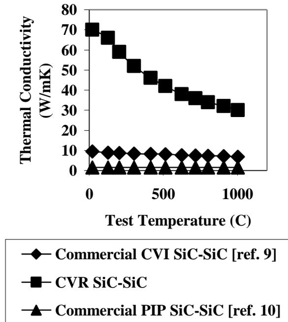
**Figure 6. Thermal conductivity of CVR-SiC/CVR-SiC composite.**
