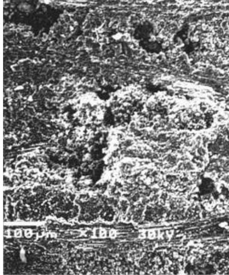
**Figure 1. Cross-section of SiC-SiC composites made with T-300 1K plain weave fabric: 4 mm thick.**
