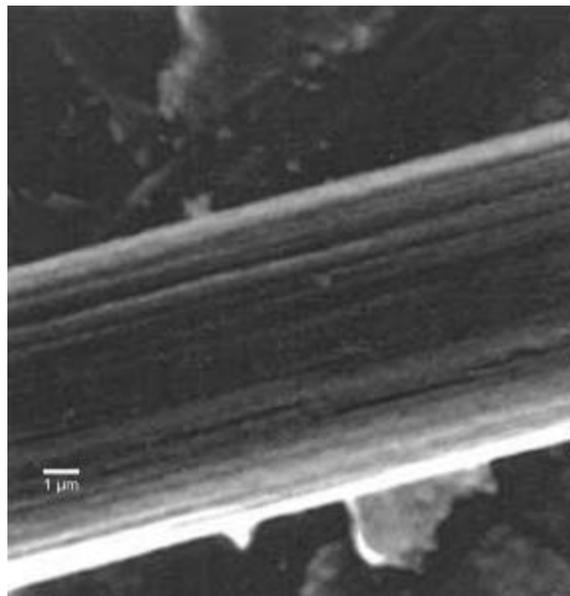
**Figure 4. SEM micrograph of 90% CVR-SiC fibers.**
