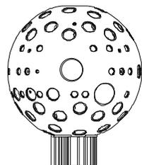
**Fig. 2 NIF chamber 10 m dia 150 tons.**
