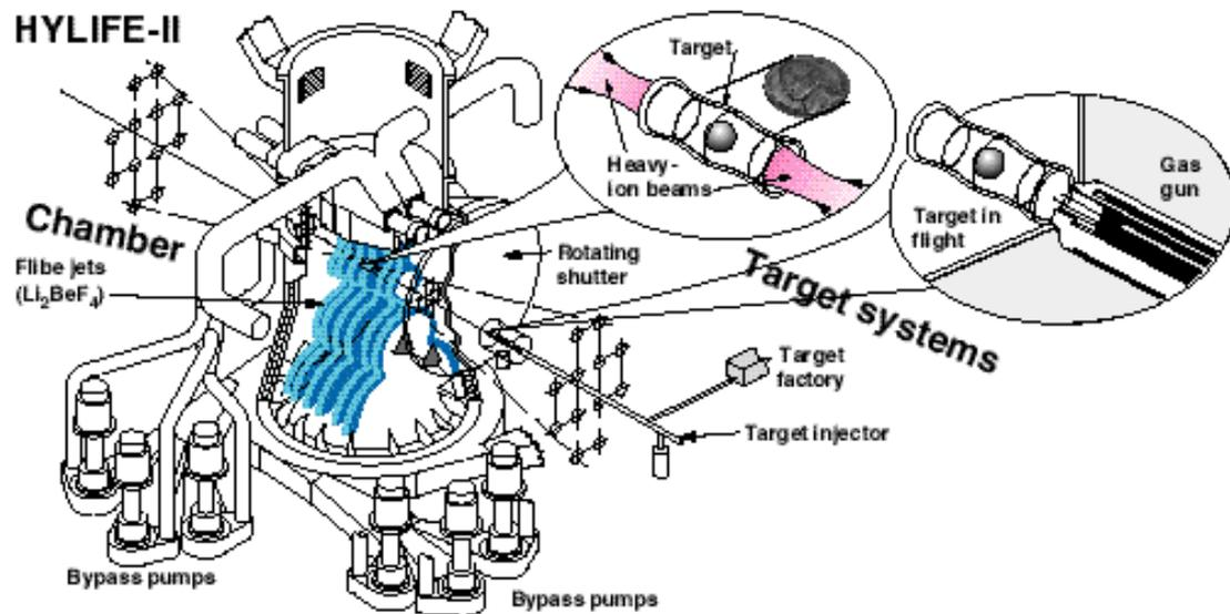
Fig. 1 HYLIFE-II chamber 7 m dia 208 tons
